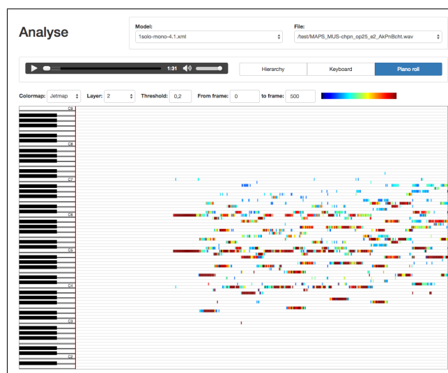
Figure 1. Piano roll visualization with integrate audio player. The type of observed features, threshold and colormap can be dynamically modified.
